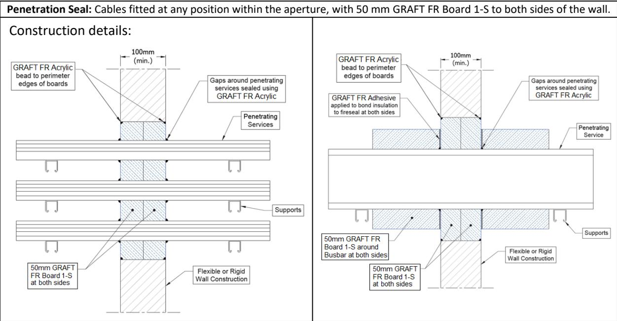
**A.6.1.1 Double side penetration seal with electrical services**
