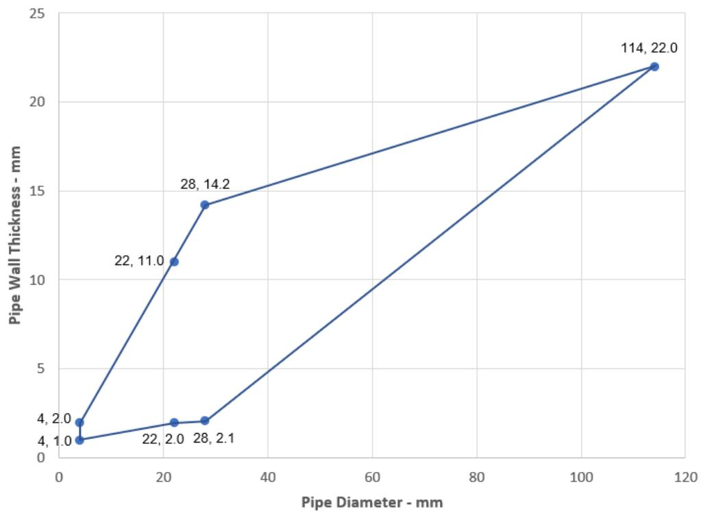
**Mild or Stainless Steel Pipes with Glass Wool Insulation - EI 60 C/U**
