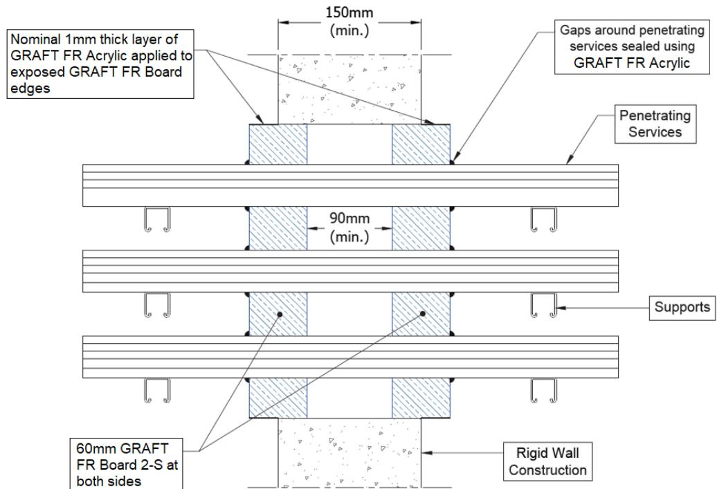
**A.1.7.1 Two side penetration seal with cables**
