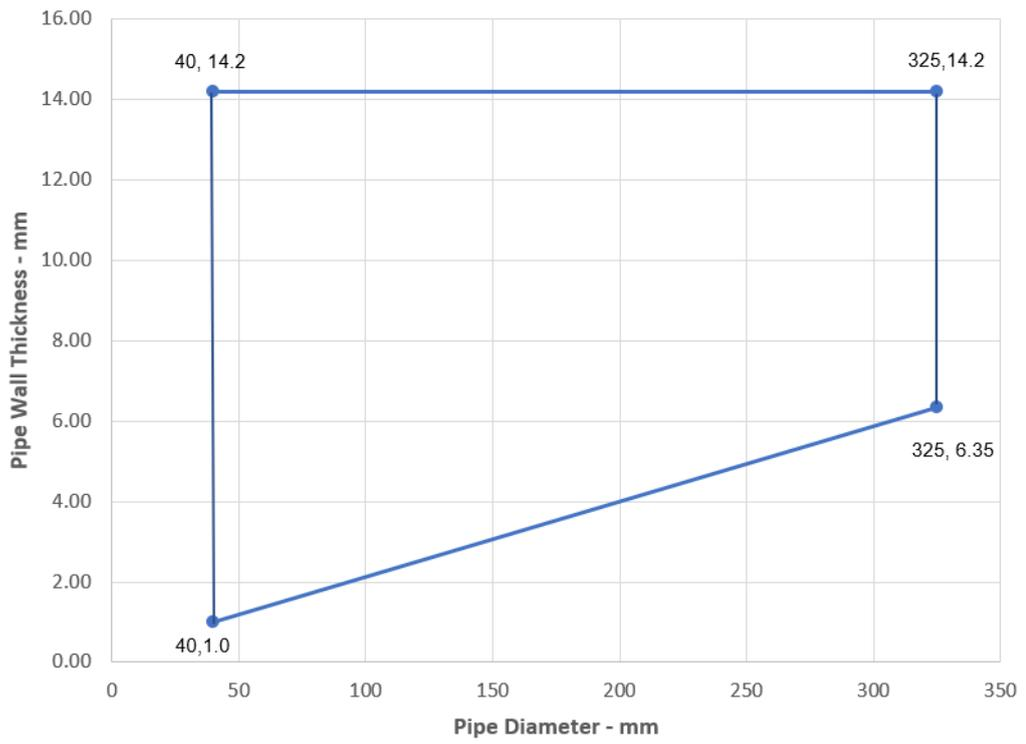
**A.1.7 GRAFT FR Board 60 mm 2-S penetration seal (protruding) blank and with cables, in rigid wall min. 150 mm thick**
