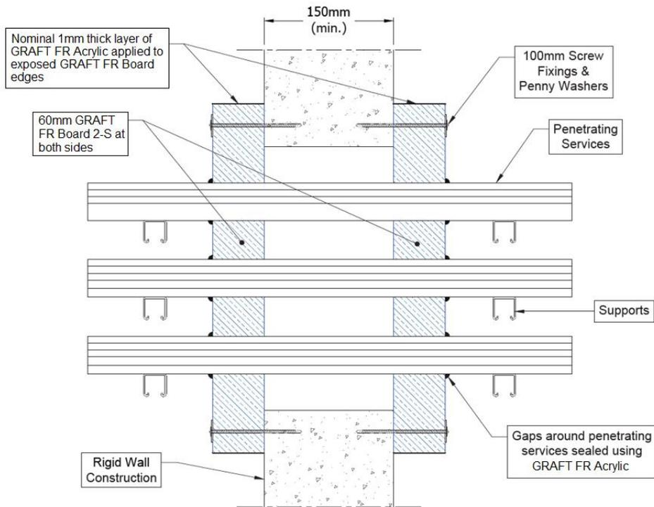
**A.1.8.1 Two side penetration seal with cables**
