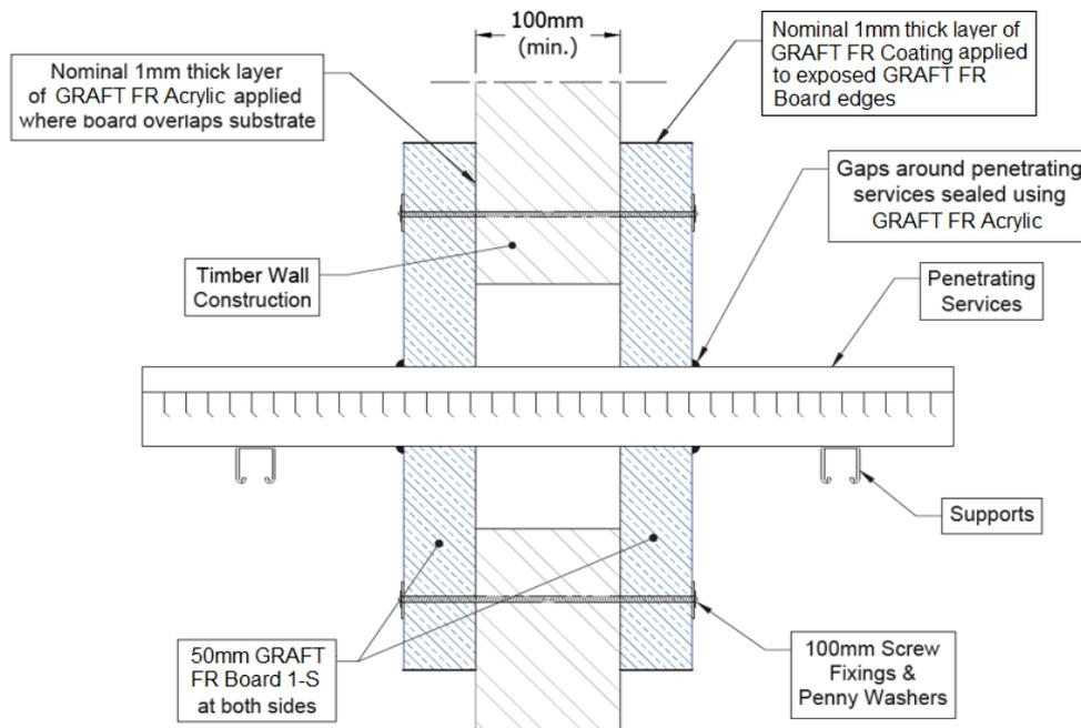
**A.8.1.1 Two side penetration seal with cables**
