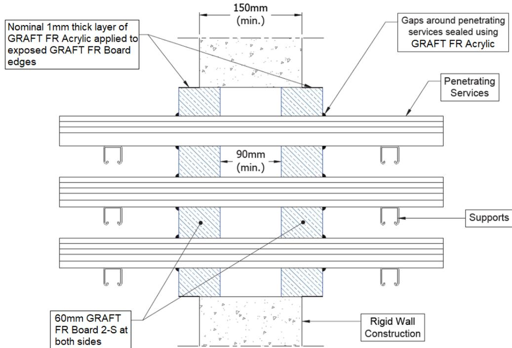
**A.1.7.1 Two side penetration seal with cables**
