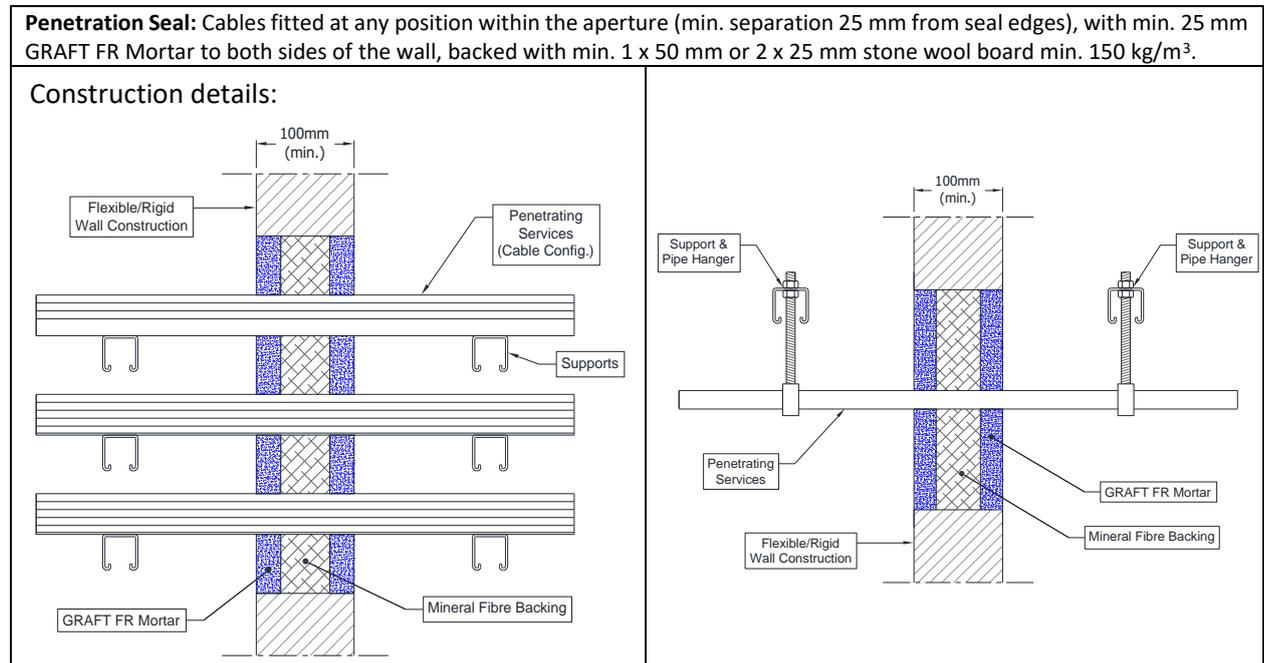
**A.5.1.1 Double side penetration seal with cables**
