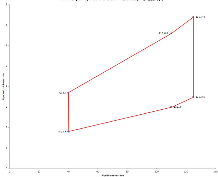
PE pipes U/C with Graft FR Pipe Wraps - EI 120 U/C
