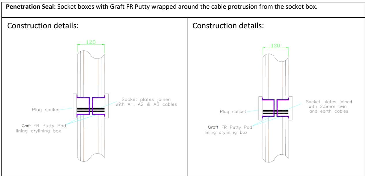
**A.2.1.1 Double side penetration seal with cables in socket boxes**
