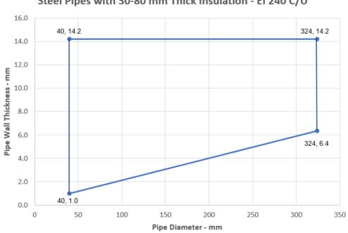
Copper or Steel Pipes with 30-80 mm Thick Insulation EI 240 C/C
