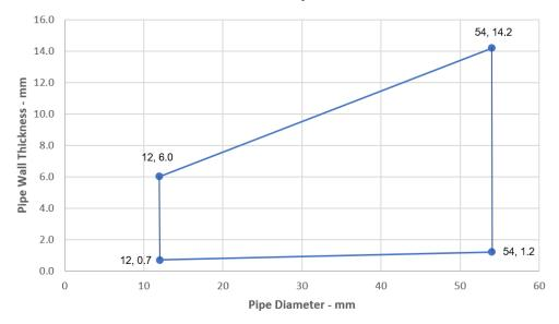
Steel Pipes with 30-80 mm Thick Insulation - EI 240 C/U
