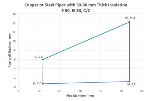
Steel Pipes with 30-80 mm Thick Insulation- E 90, El 60, C/U
